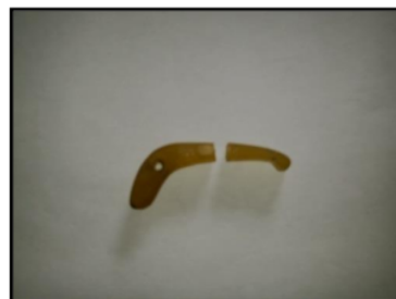
Figure 5. There is an unequal stress concentration due to the influence of the handle design
