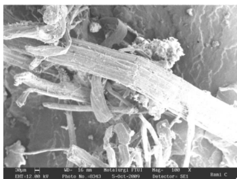
Figure 13. SEM Photo Fracture analysis begins with a matrix crack on the surface of the Polypropylene matrix composite
