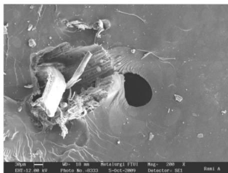
Figure 12. SEM image showing fracture analysis begins with cracked ramie fibers (fibers released from the matrix) on the surface of the epoxy composite matrix
