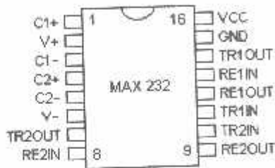
Above: (Figure 6) Pinouts for the MAX-232, RS-232 Driver/Receiver.
