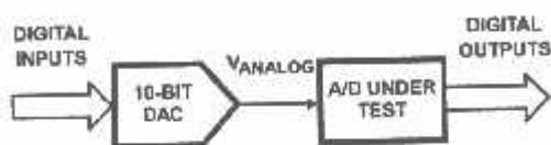
FIGURE 20. BASIC "DIGITAL" A/D TESTER
