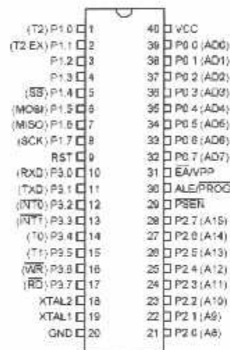
Gambar 2.5 Konfigurasi Pin-Pin AT89S8252
