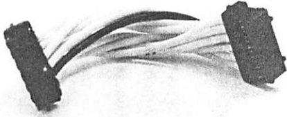
12pin Cable (Connecting EG-SR-7150MJ to Test Board)
