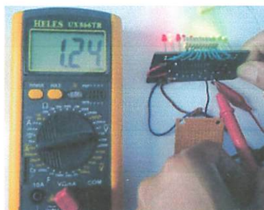
Gambar 4.4 Pengujian Bar/Dot Display Driver
