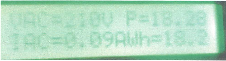
Gambar 4.6 Monitoring Berbeban 1 Lampu Bolam
