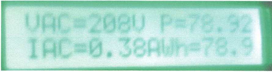
Gambar 4.7 Monitoring Berbeban 2 Lampu Bolam
