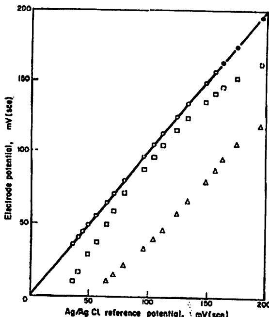
FIG. 5. Comparison of potentials of electrodes which had been exposed to I<sup>-</sup> with those of a nominally pure Ag/AgCl electrode.
