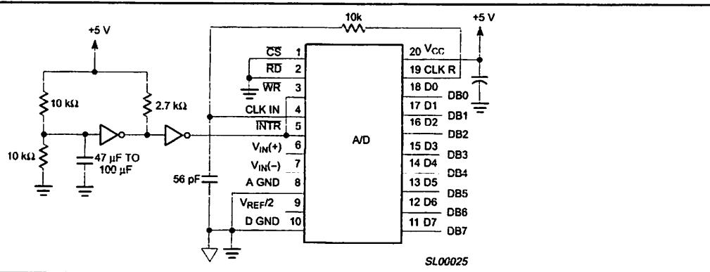
Figure 10. Connection for Continuous Conversion
