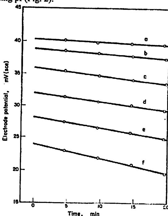
FIG. 2. Relations of electrode potential to time in solutions of pCl 1 and six values of pH. The straight lines drawn are least squares fit to the data. The pH values and slopes (mV/min) for each curve are: a, 3.54, -0.04; b, 3.42, -0.07; c, 3.26, -0.12; d, 3.14, -0.13; e, 3.05, -0.16; f, 2.98, -0.22. Each point represents the average of potentials of 8 electrodes.
