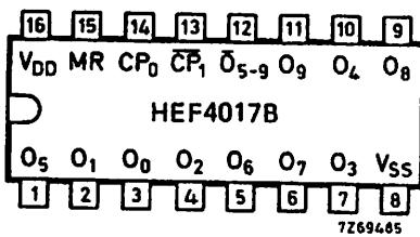
Fig.2 Pinning diagram.
