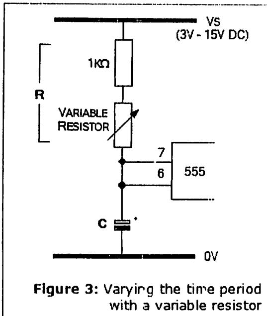
**Figure 3:** Varying the time period with a variable resistor
