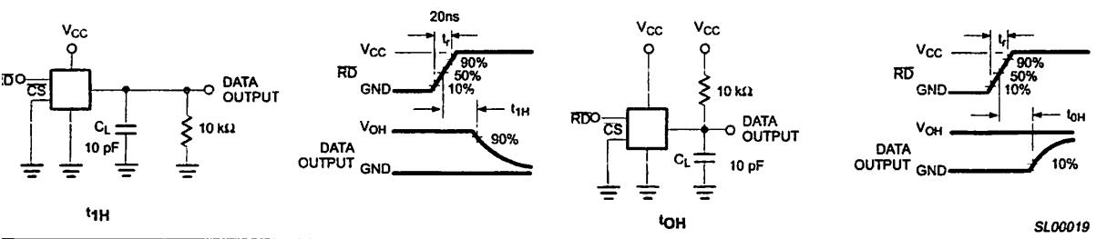
Figure 4. 3-State Test Circuits and Waveforms (ADC0801-1)
