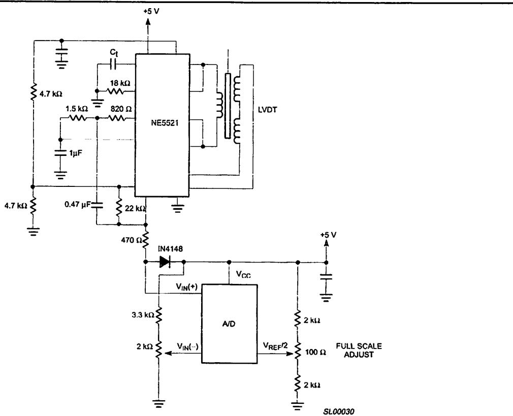
Figure 15. Digitizing a Transducer Interface Output
