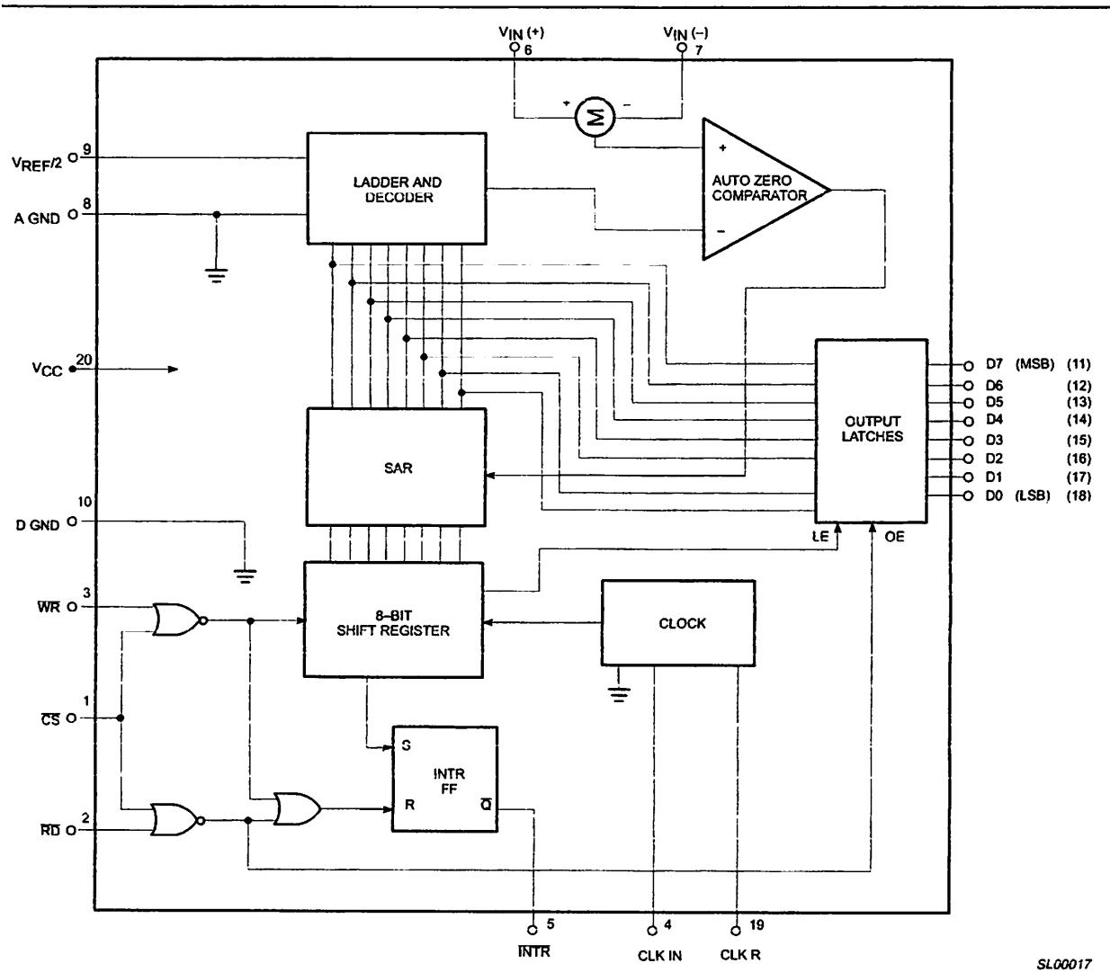
Figure 2. Block diagram
