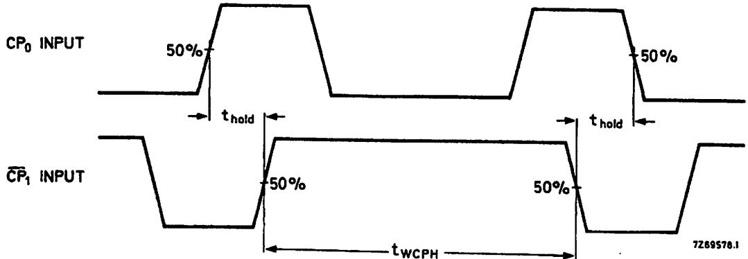
Fig.4 Waveforms showing hold times for CP<sub>0</sub> to CP<sub>1</sub> and CP<sub>1</sub> to CP<sub>0</sub>. Hold times are shown as positive values, but may be specified as negative values.
