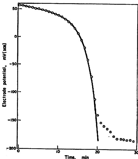
FIG. 4. Electrochemical transformation of the same electrode as in Fig. 3. The circles are potentials determined by digital voltmeter every 50 s during the interval shown. The solid line is a plot of
