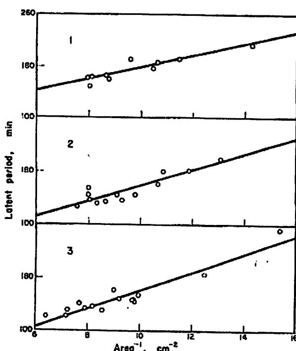
FIG. 6. Relation of the latent period of transformation to the reciprocal of electrode area. Each point represents data for a single electrode. The numbers 1, 2 and 3 correspond to the pCl values for each set of points. The straight lines were fitted by the least squares method to the data, and have slopes of 9.0, 11.8, and 13.8 min . cm<sup>2</sup> for pCl values of 1, 2 and 3 respectively.
