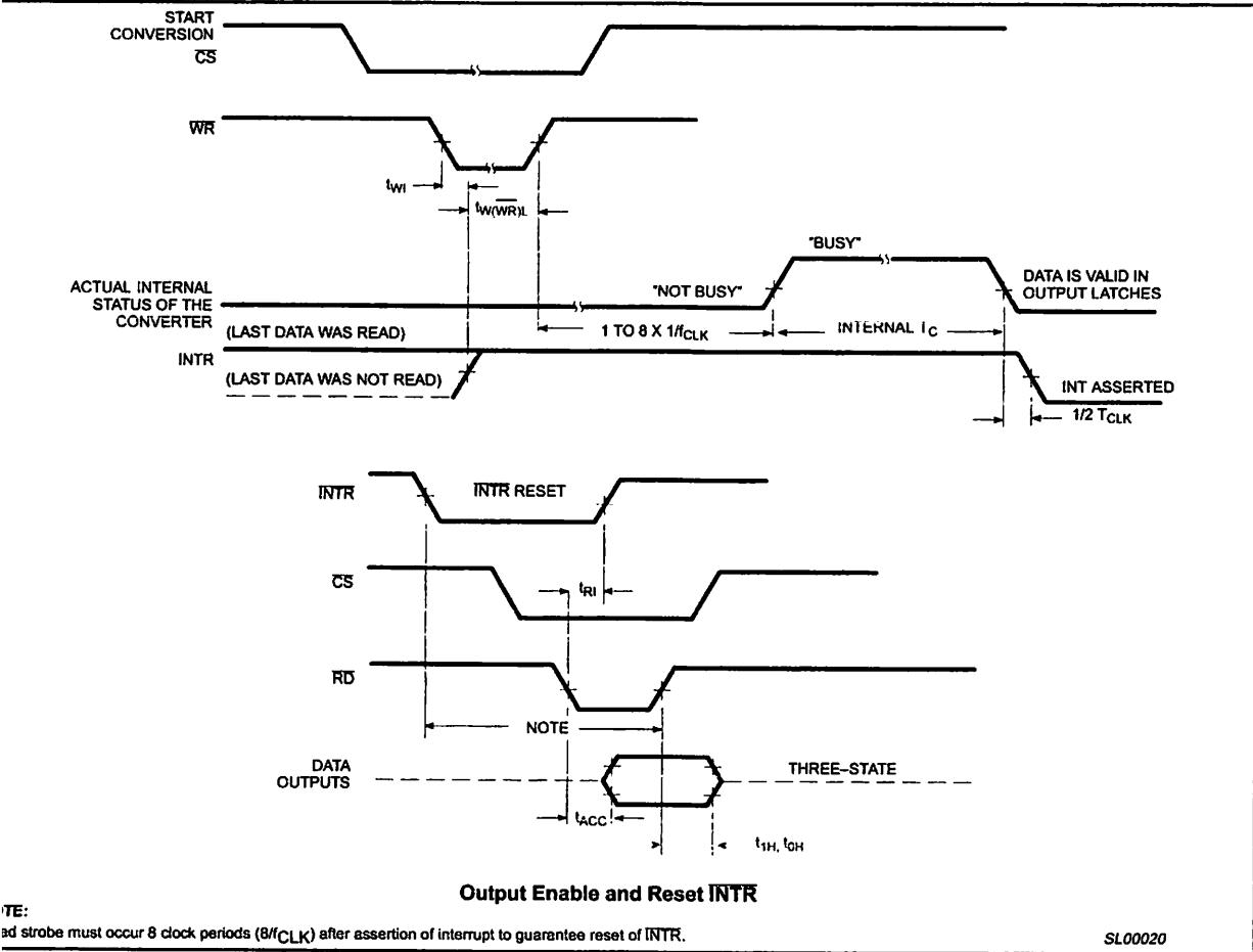
Figure 5. Timing Diagrams
