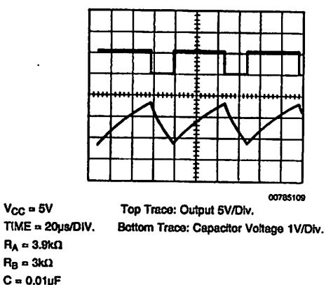
**FIGURE 5. Astable Waveforms**
