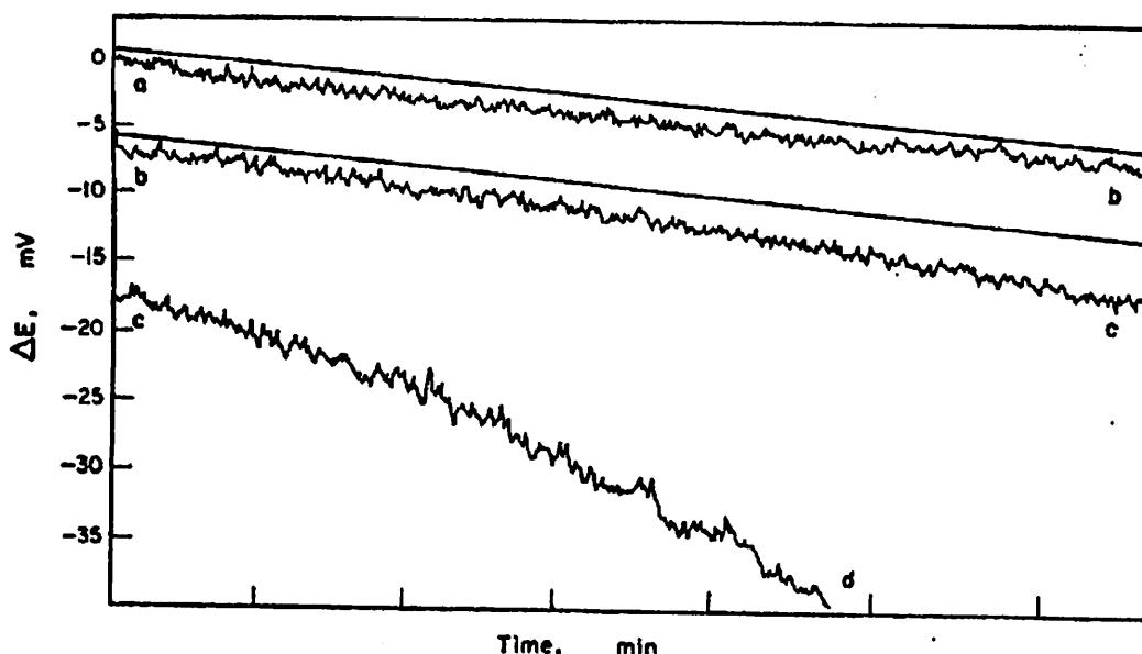
FIG. 3. Analogue record of a single electrode potential change with time, illustrating oscillation of the potential.
