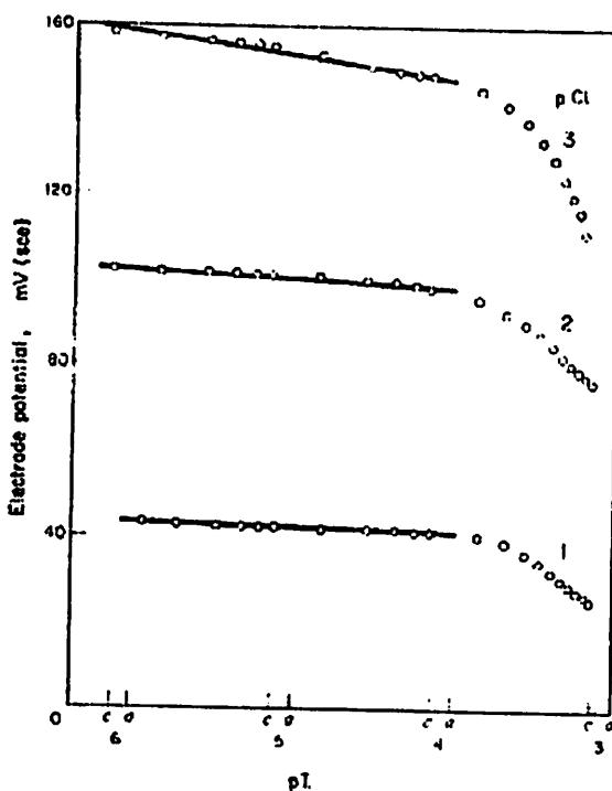
FIG. 1. Relations of electrode potential to pH for 3 pCl values.
