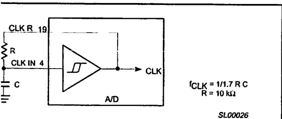
Figure 11. Self-Clocking the Converter
