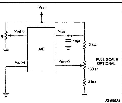
Figure 9. Ratiometric Mode of Operation with Optional Full Scale Adjustment
