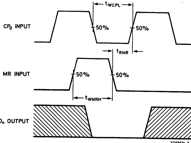
Conditions: CP<sub>1</sub> = LOW while CP<sub>0</sub> is triggered on a LOW to HIGH transition. t<sub>WCPL</sub> and t<sub>RMR</sub> also apply when CP<sub>0</sub> = HIGH and CP<sub>1</sub> is triggered on a HIGH to LOW transition.
