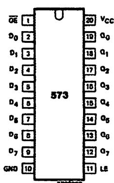
Fig.1 Pin configuration.
