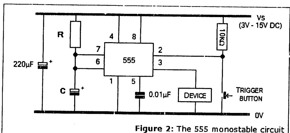
Figure 2: The 555 monostable circuit
