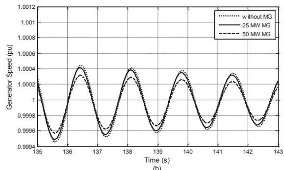
Fig. 3. Speed of generator 2 (a) and 4 (b) for three phase fault at bus 7.
