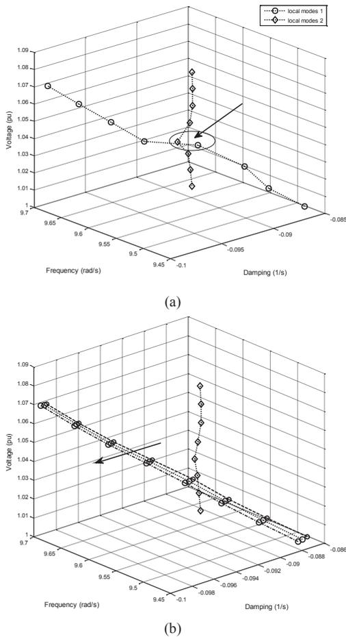
Fig. 5. Local modes trajectories near weak resonance without (a) and with (b) MG penetration.
