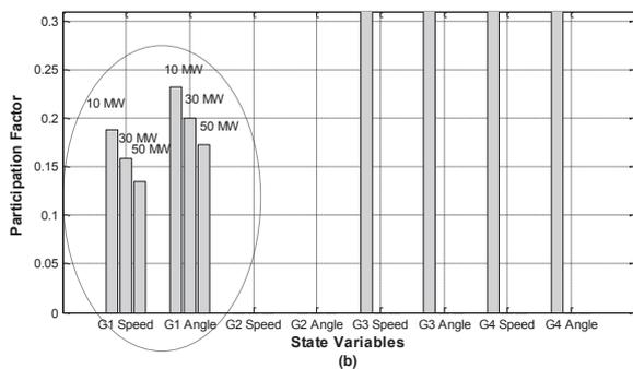
Fig. 7. Local modes 1 (a) and 2 (b) participation factor near weak resonance with increased MG penetration.
