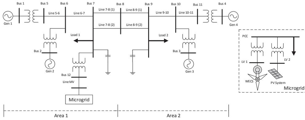
Fig. 1. Two-Area Four Generators System with Microgrid.
