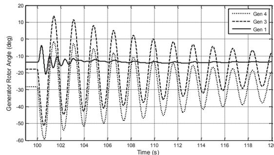
Fig. 4. Rotor angle of generator 1, 3 and 4 for three phase fault at bus 7.
