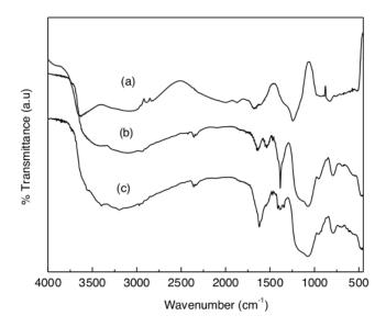
Figure 1. Spectrum FTIR sample (a) silica; and silica prepared using acid (b) HCl; (c) H<sub>2</sub>SO<sub>4</sub>
