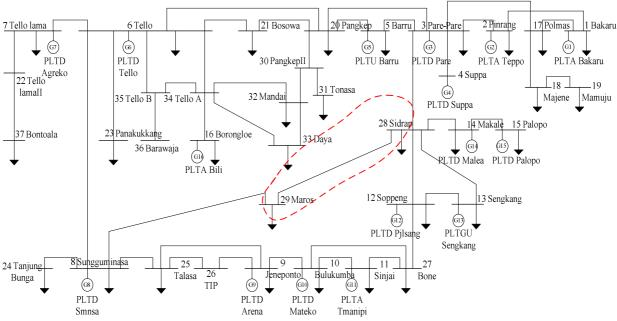
Figure 6. One-Line Diagram of the Sulselrabar Multimesin
