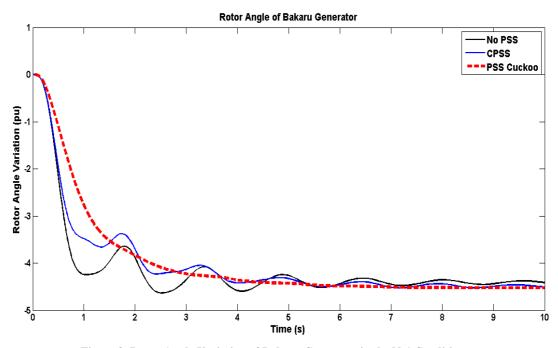
Figure 8. Rotor-Angle Variation of Bakaru Generator in the N-1 Condition
