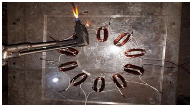
Fig. 11 The winding to the stator installed permanently.
