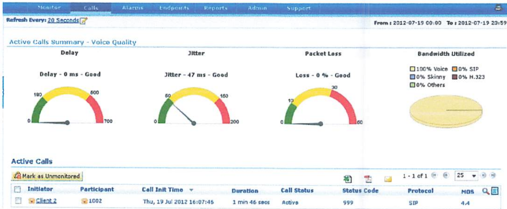
Gambar 4.23 Monitoring Voice Quality Client 2 Ke Ekstensi 1002
