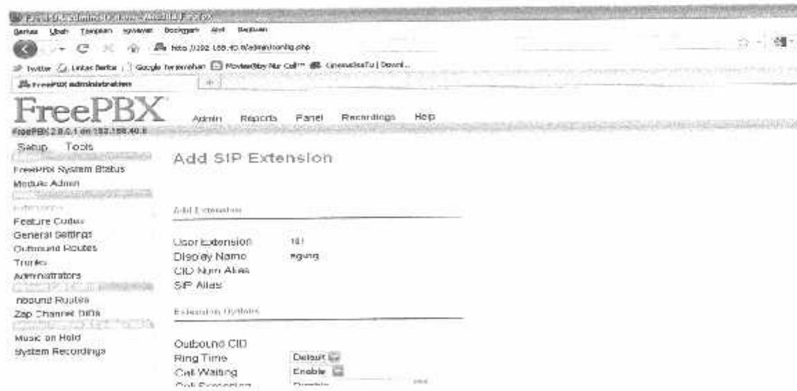
Gambar 4.10 Tampilan Add SIP Extension Pada Kolom Add Extension
