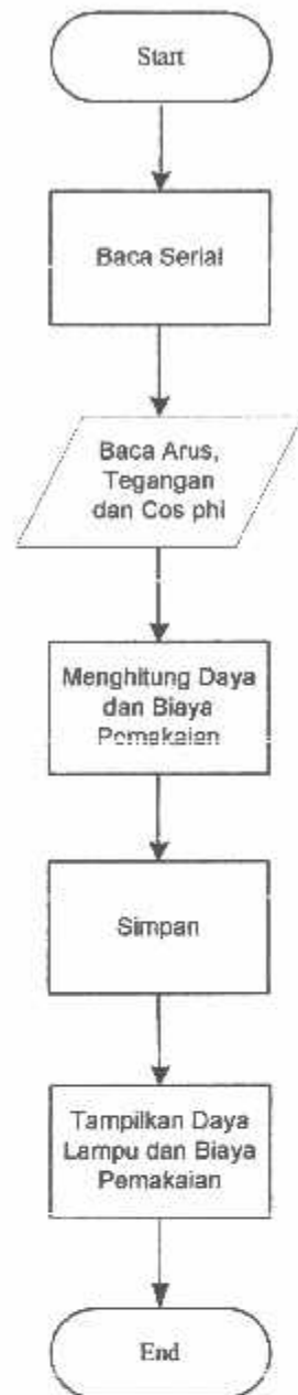
Gambar 3.2 Diagram Alir Program Monitoring
