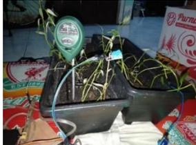
Gambar 4.14 Pengujian Sensor *Soil Moisture*
