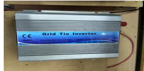
Gambar 2.8 GTI ( Grid Tie Inverter )
