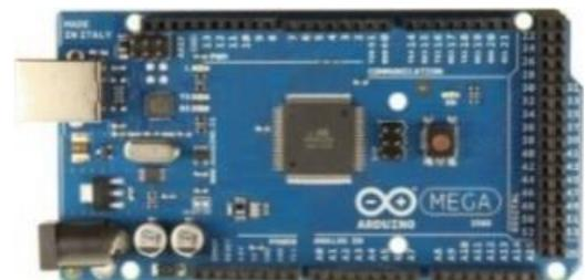
Gambar 6 Board Arduino Mega 2560
