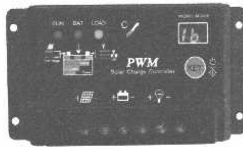
Gambar 2.8 Solar Charge Control
