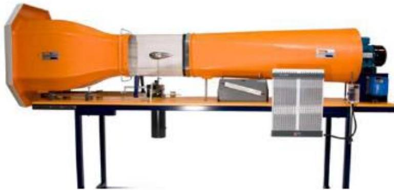
Gambar 2.7 *Wind tunnel*
