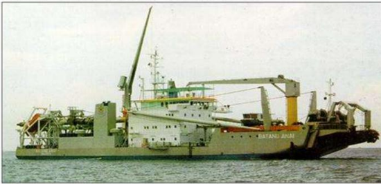
CUTTER SUCTION DREDGER BATANG ANAI
