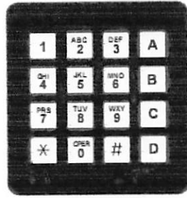
Gambar 2.18 Keypad Matrik 4 x 4 (Sumber: Data Sheet Keypad)
