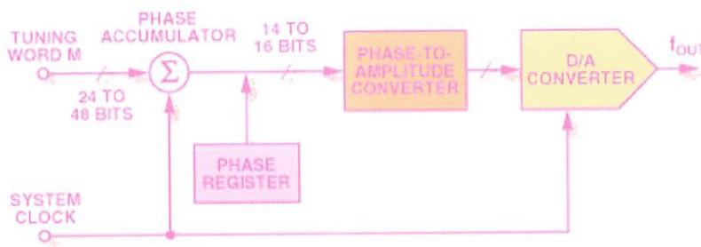
**Figure 3. Components of a direct digital synthesizer.**
