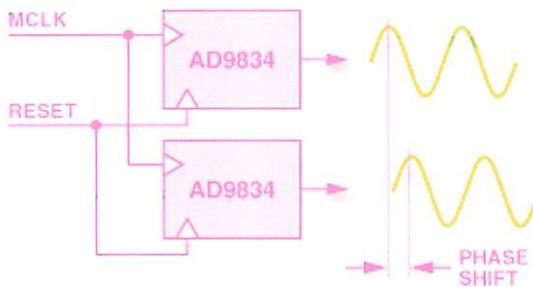
**Figure 8. Multiple DDS ICs in synchronous mode.**
