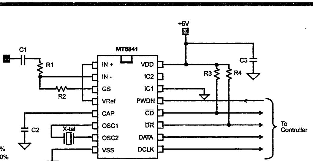
Figure 6 - Application Circuit (Single-Ended Input)
