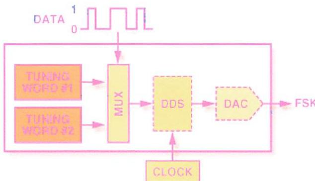
**Figure 7. A DDS-based FSK encoder.**
