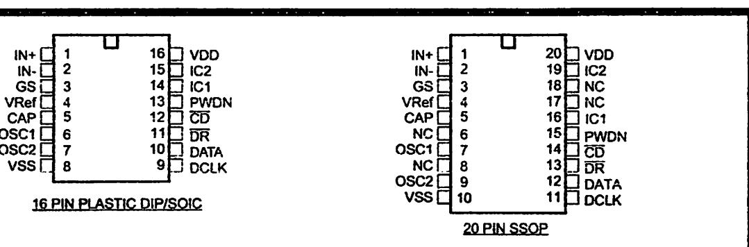
Figure 2 - Pin Connections
