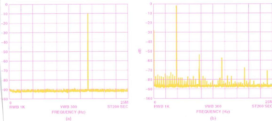
**Figure 10. Output of an AD9834 with a 50-MHz master clock and**
