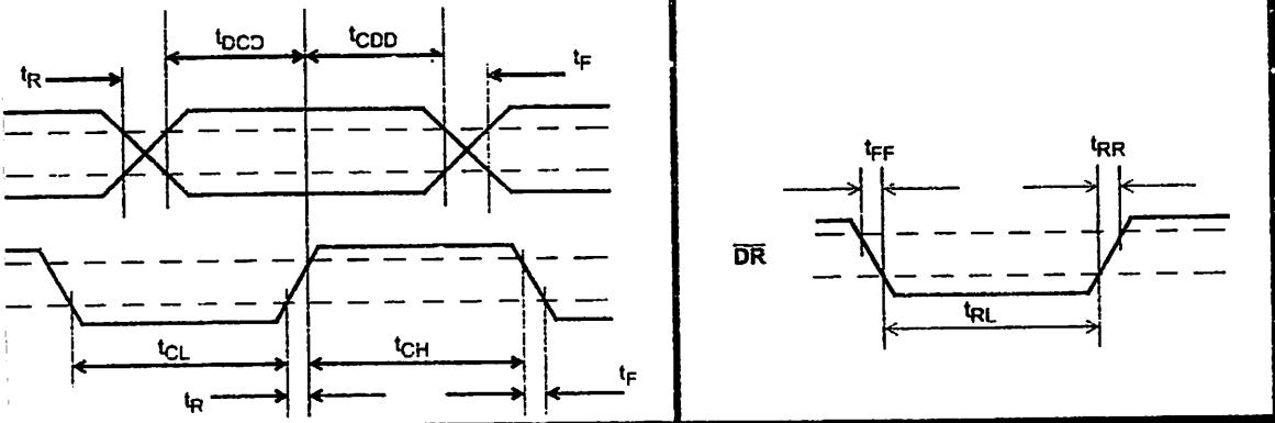
Figure 7 - DATA and DCLK Output Timing
