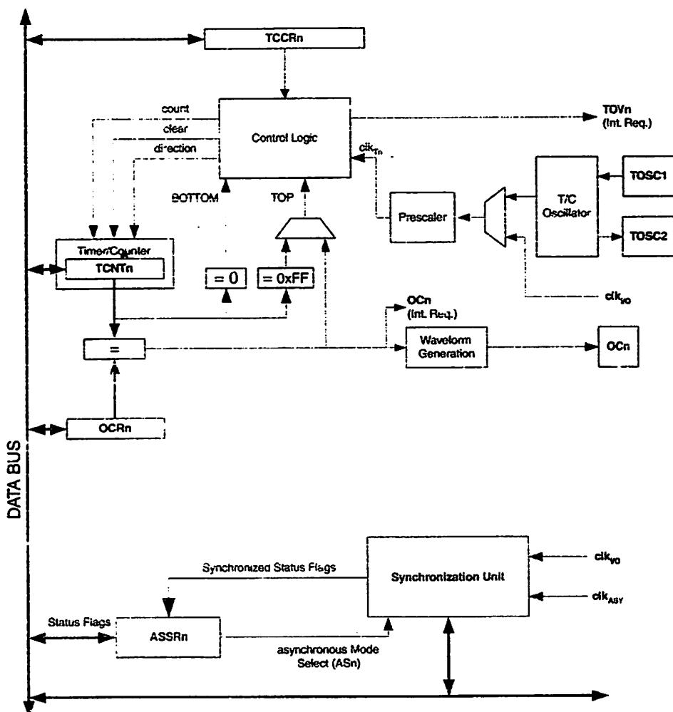
The Timer/Counter (TCNT2) and Output Compare Register (OCR2) are 8-bit registers. Interrupt request (shorten as Int.Req.) signals are all visible in the Timer Interrupt Flag Register (TIFR). All interrupts are individually masked with the Timer Interrupt Mask Register (TIMSK). TIFR and TIMSK are not shown in the figure since these registers are shared by other timer units.
