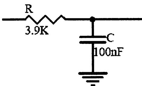
Gambar 2.12. Rangkain Low Pass Filter<sup>[4]</sup>
