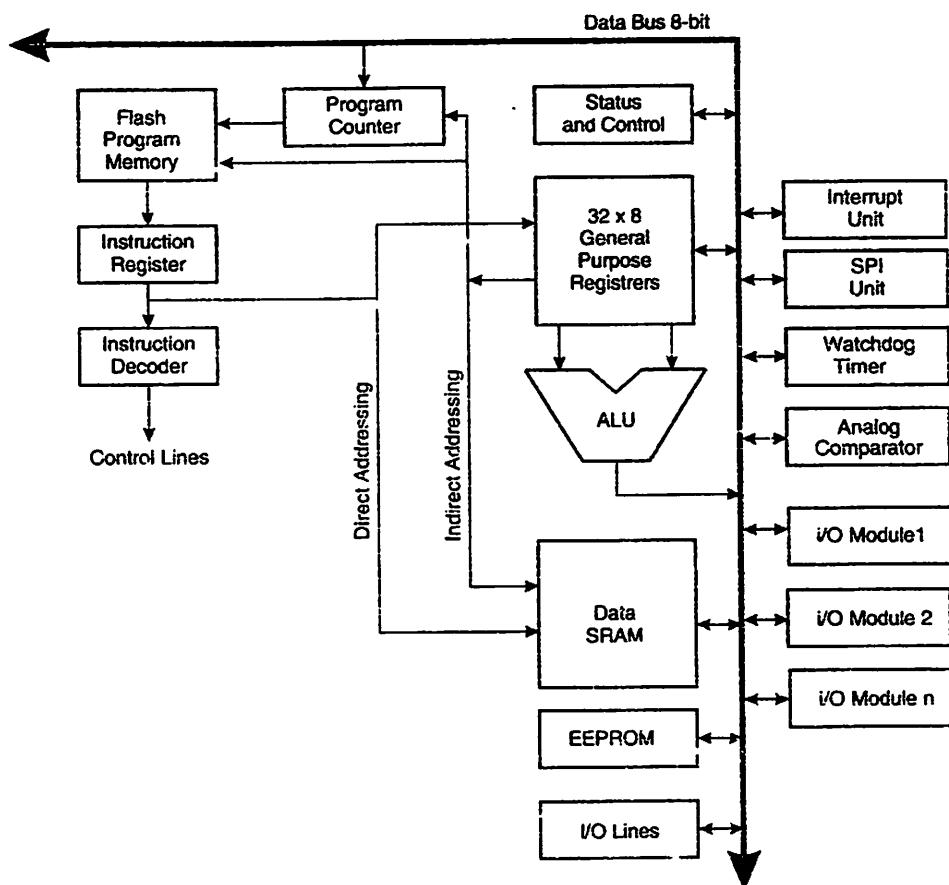
In order to maximize performance and parallelism, the AVR uses a Harvard architecture – with separate memories and buses for program and data. Instructions in the Program memory are executed with a single level pipelining. While one instruction is being executed, the next instruction is pre-fetched from the Program memory. This concept enables instructions to be executed in every clock cycle. The Program memory is In-System Reprogrammable Flash memory.
