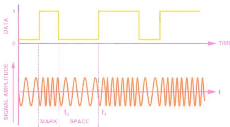
**Figure 6. FSK modulation.**
