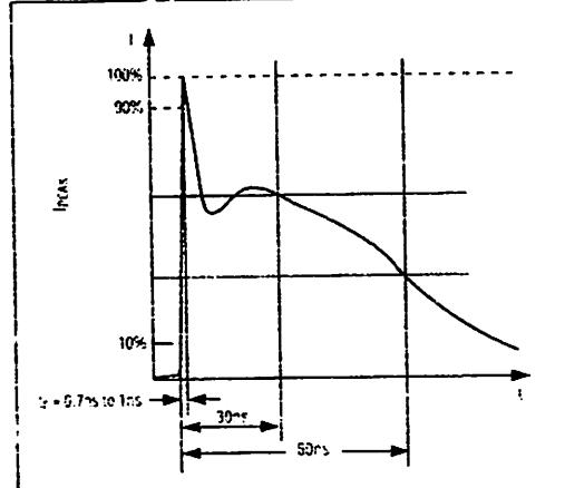
Figure 7b. IEC1000-4-2 ESD Generator Current Waveform
