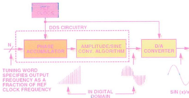
**Figure 5. Signal flow through the DDS architecture.**
