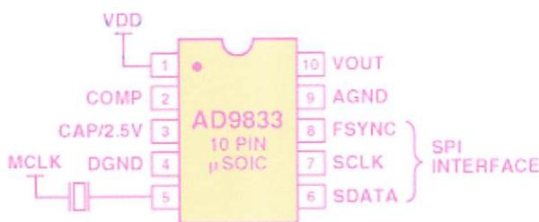
Figure 1. The AD9833—a one-chip waveform generator.
