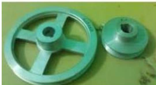
**Gambar 2. 12 *Pulley Tipe A***
