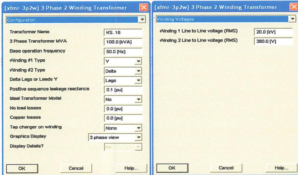
Gambar 3.13 Tampilan Input Data Transformator
