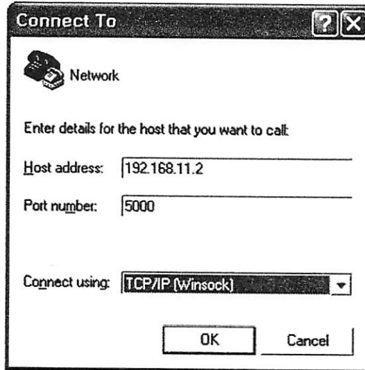
Figure 34. Network Terminal Program configuration
