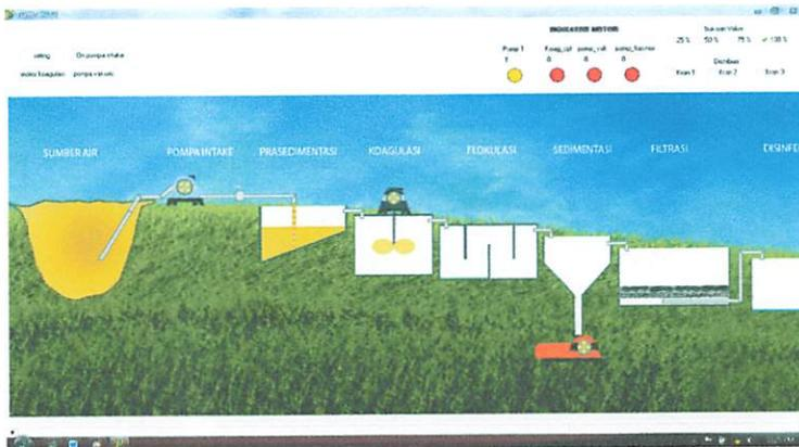
Gambar 4.37 Kondisi Pengoprasian Pompa Intake Saat Intruksi Push Button On Pompa Intake Ditekan
