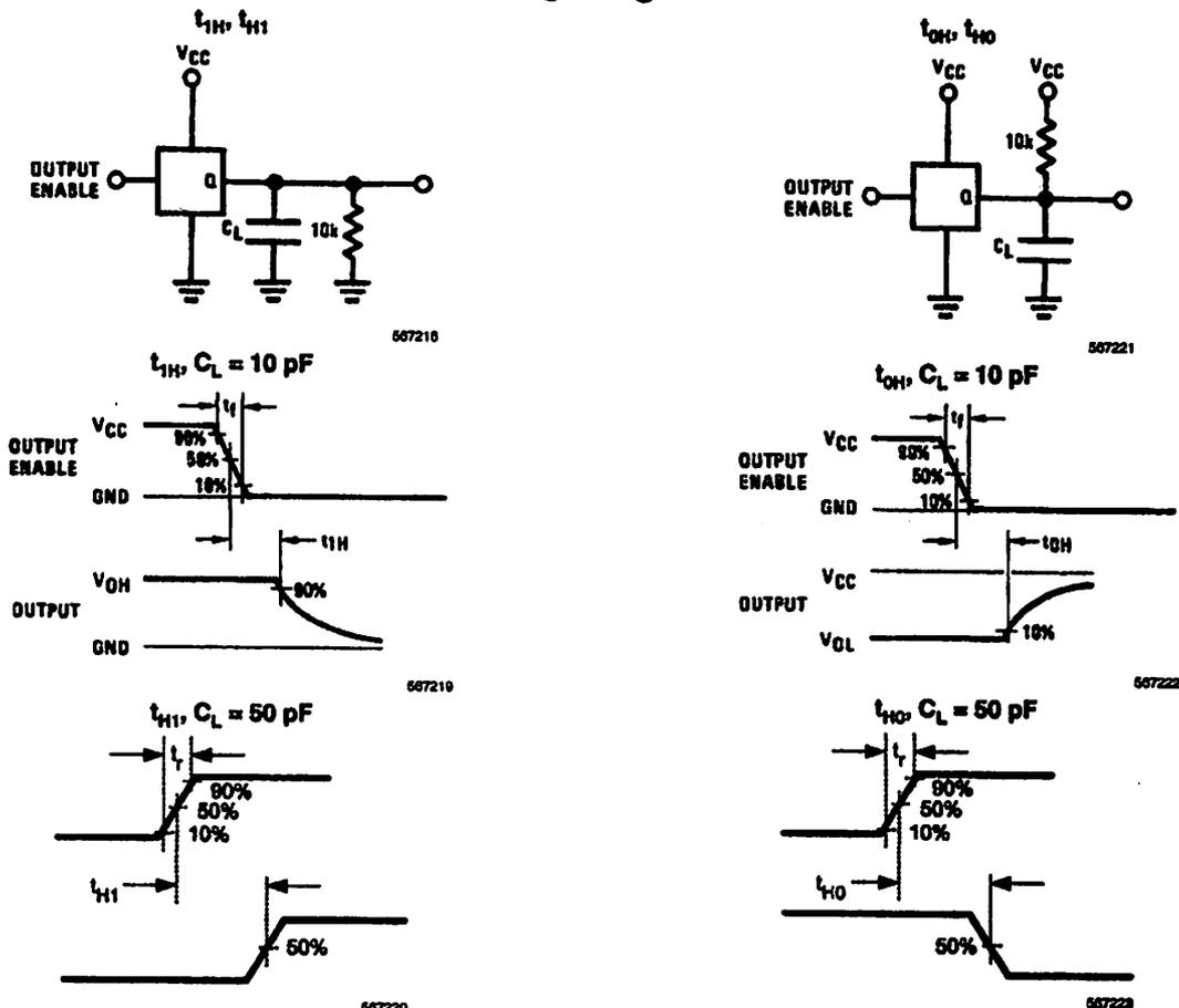
FIGURE 8. TRI-STATE Test Circuits and Timing Diagrams
