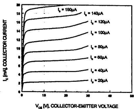
Figure 1. Static Characteristic
