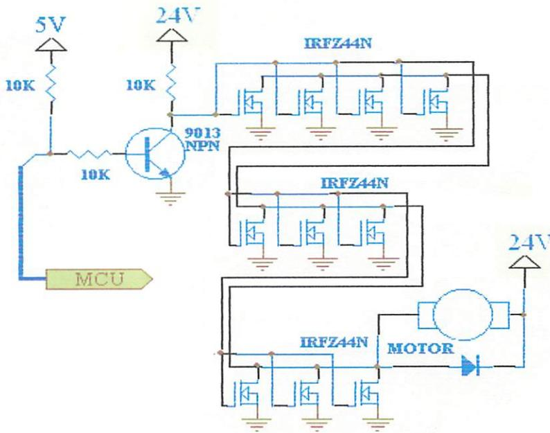
Gambar 3.10 Rangkaian Driver Motor
