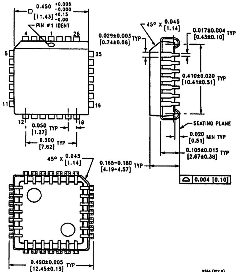
Molded Chip Carrier (V)
