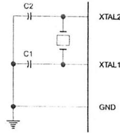
Note: C1, C2 = 30 pF ± 10 pF for Crystals = 40 pF ± 10 pF for Ceramic Resonators
