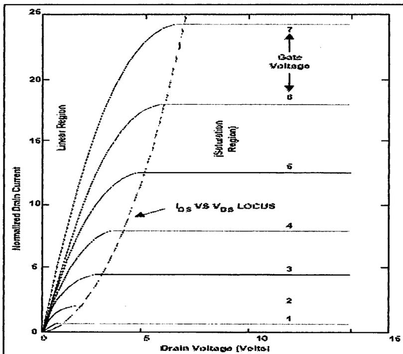
**Gambar 2.14** Current-Voltage Characteristic<sup>[10]</sup>
