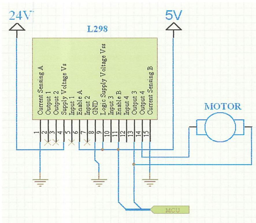
Gambar 3.13 Rangkaian Driver Motor Dua Arah On/Off
