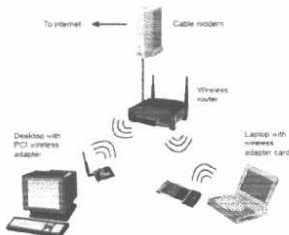
Gambar 2.2 Sistem Wireless Local Area Network
