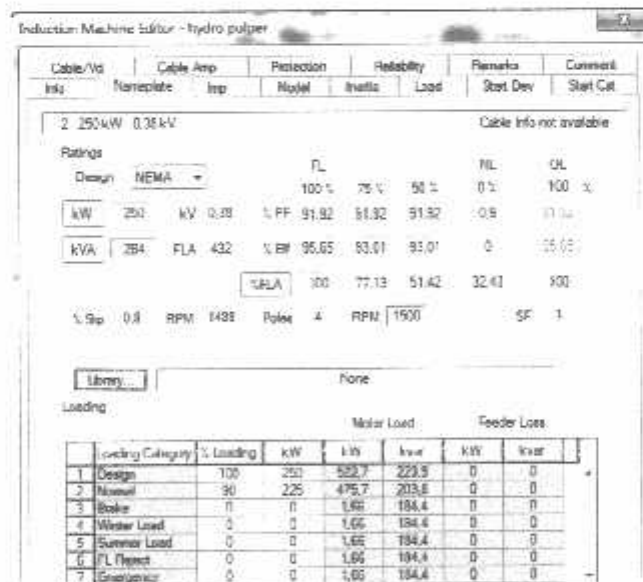
Gambar 4.2 Inputan Data Name Plate Motor kedalam Software ETAP Powerstation
