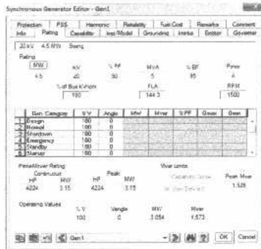
Gambar 3.5 Input Rating Generator di ETAP Powerstation
