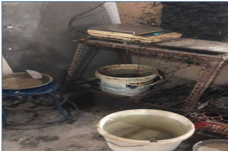
Penimbangan Didalam Air Benda Uji
