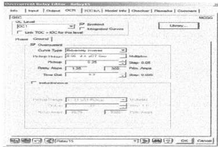
Gambar 4.9 Input Parameter Setting Awal Relay 15 GFR ( ground fault relay ) Tipe MCGG
