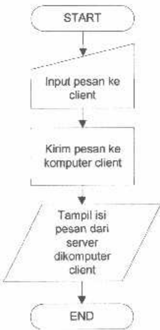
Gambar 3.5 Flowchart proses kirim pesan ke client
