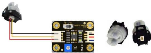
Gambar 2.4 Modul Sensor Turbidity
