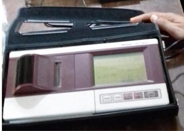
Gambar 3.7 Surface Roughness Tester
