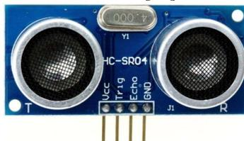
Gambar 5. Sensor ultrasonik
