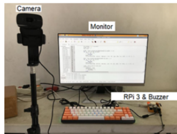
Figure 5. Face mask detector hardware
