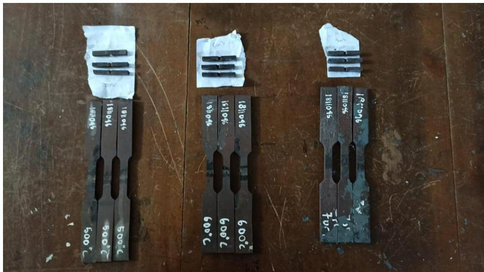
**Gambar 3.20. Spesimen Sesudah Proses Heat Treatment Annealing**
