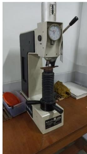
**Gambar 3.21. Rockwell Hardness**
