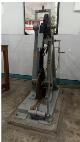
**Gambar 3.23. Alat Uji Impak**
