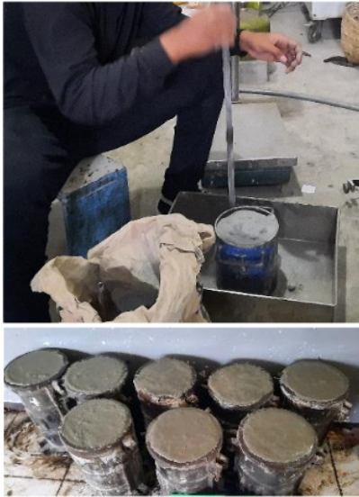
Fig.2 The molding process of concrete materials
