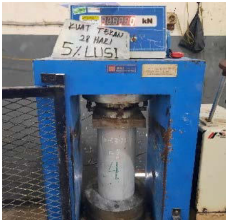
Fig.5 Concrete compression machine
