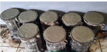
Fig.4 Wet concrete mixes are left for 28 days.
