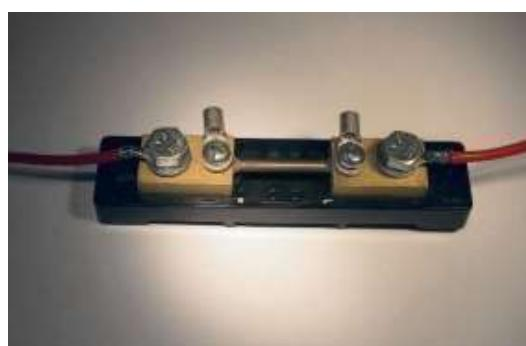
2.3 Gambar “Resistor Shunt”
