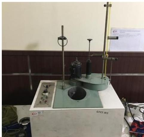
**Gambar 2.7 Bomb calorimeter**
