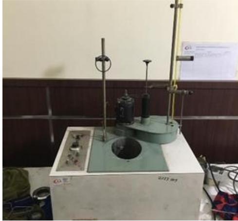
**Gambar 3.9 Bomb calorimeter**
