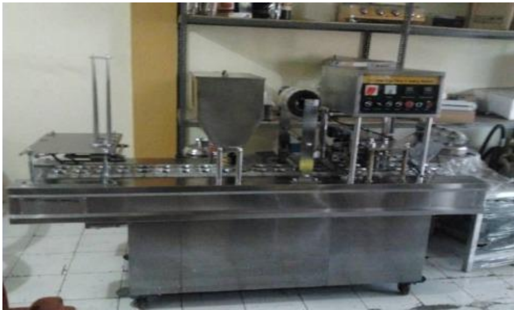
Gambar 1.1 Gambar Mesin Cup Sealer (Sumber: UMKM Sari Apel Brosem)
