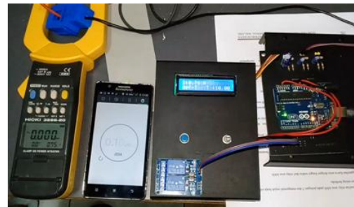
Gambar 4.6 OCR Karakteristik Definite Time Beban R1
