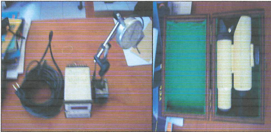
MVD Amplifier, LVDT, Crack detector
