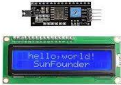
Gambar 2. 5 LCD 16x2 I2C
