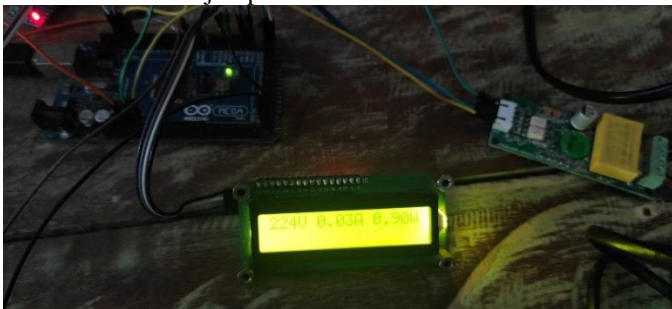
Gambar 3.4 Pengujian Sensor PZEM-004T
