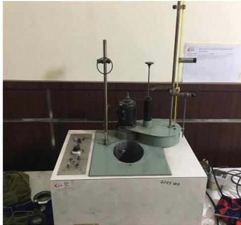
Gambar 2. 7 Bomb Calorimeter
