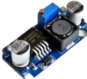
Gambar 2. 7 DC-DC step-down (buck)
